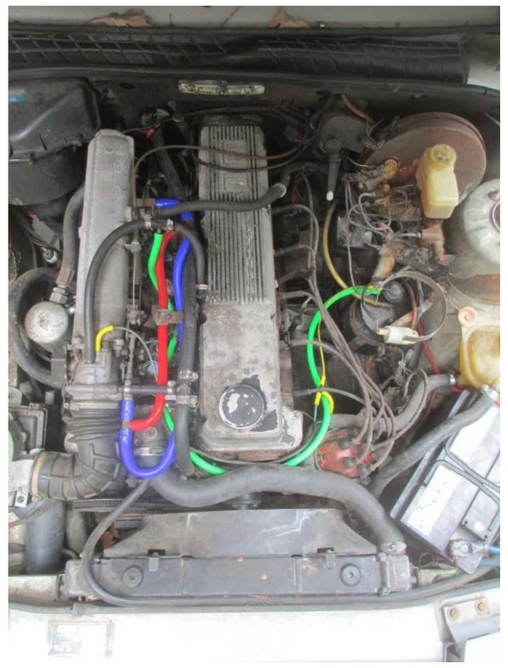
Yellow - Ignition advance and carbon canister purge valve Green - Vapour line to intake manifold
