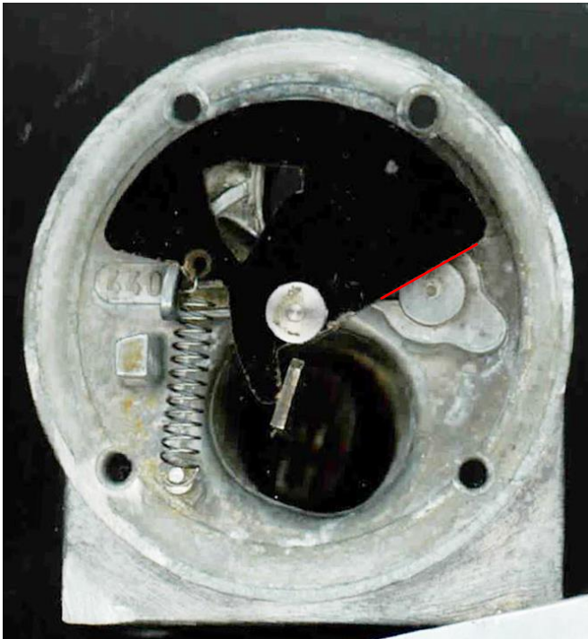
Original Bosch Spring at 17°C, 26° angle from fully closed
