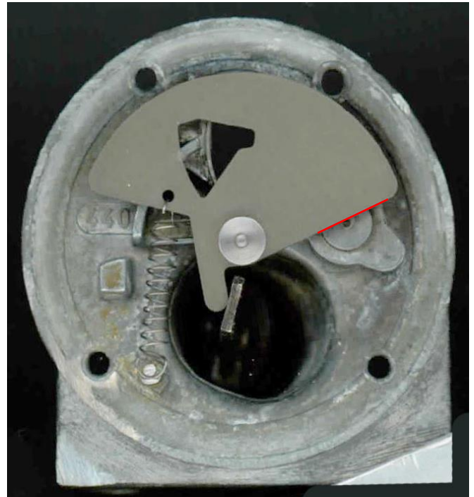
Missing Parts Spring at 17°C, 34° angle from fully closed
